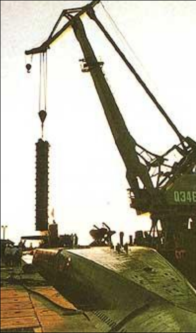
A Julang-1 SLBM is loaded into one of the Xia's 12 launch tubes.
